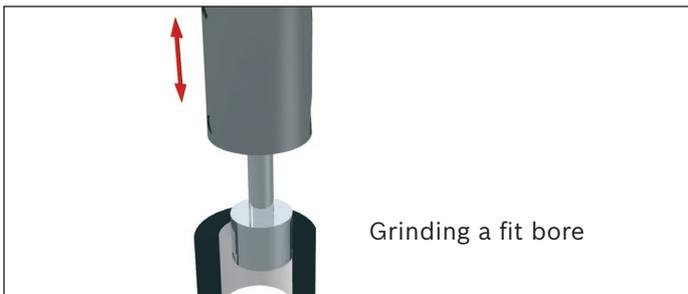
Grinding a fit bore
