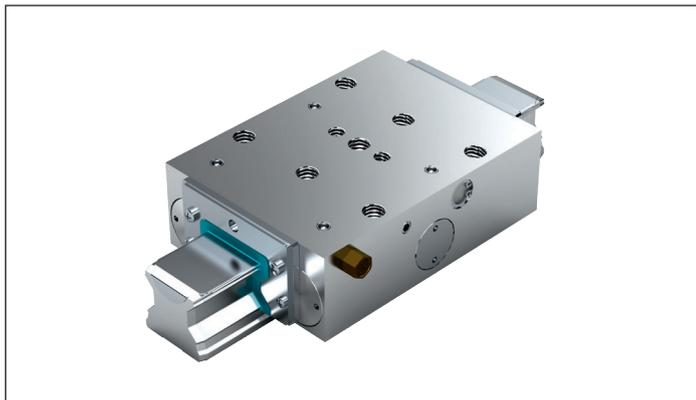
**Very high axial holding forces due to three pistons connected in series combined with strong spring energy accumulator; increased holding force thanks to additional pressure through the air-plus port.**
