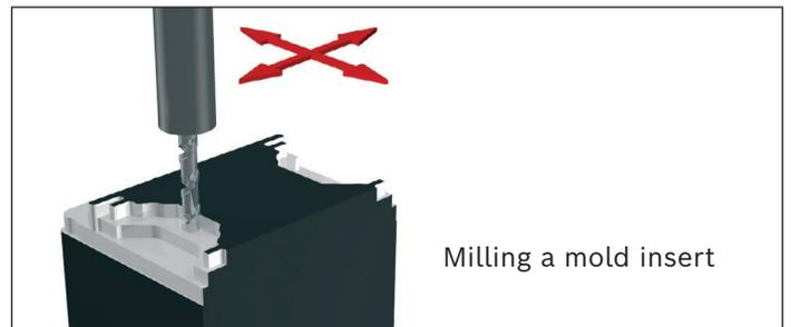
Milling a mold insert
